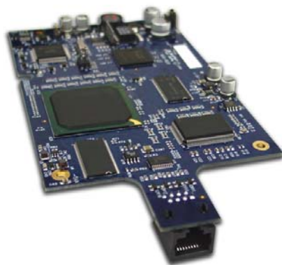
FIG. 12 NXA-RGB RGB/VGA Interface Card (installed within a VG-Series panel)
